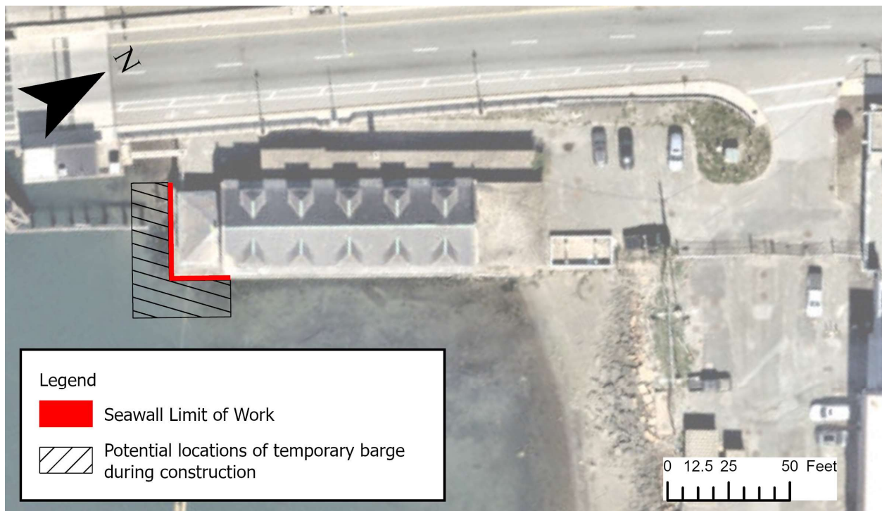
Figure 8. Potential locations of temporary barge within the Mystic River. Approximate location shown as a 15-ft buffer surrounding the 65 linear feet limits of work along the seawall.
